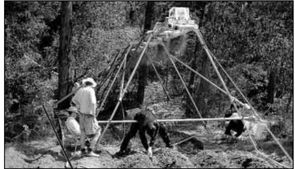
Buffer zone performance under rainfall simulator, Tarago
