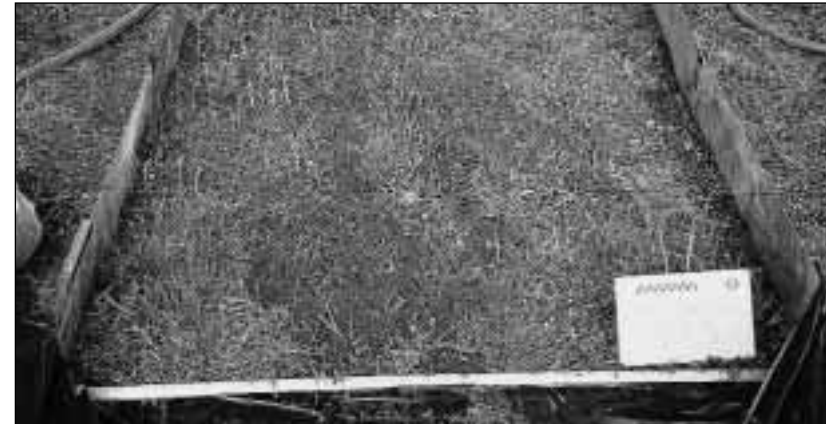
Sediment fans formed in grass filter strips in the Tarago catchment experiments.
