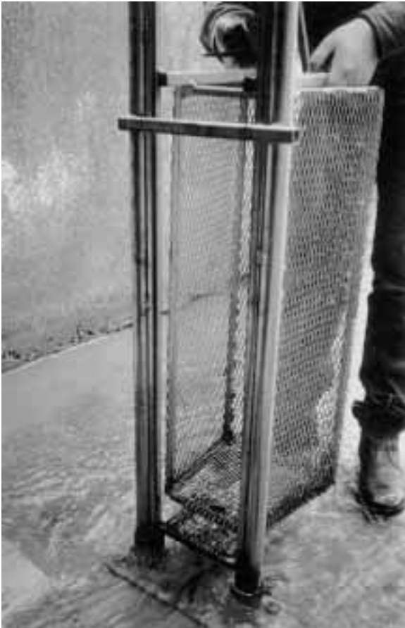
Photograph 4.2 Essery's (1994) gross pollutant sampler showing collection basket, guiding frames and base plates
