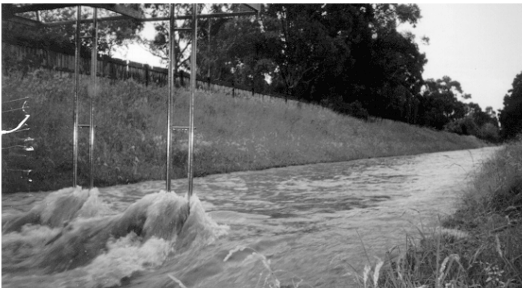
Photograph 4.1 The pilot site with materials blocking the frames during high flow
