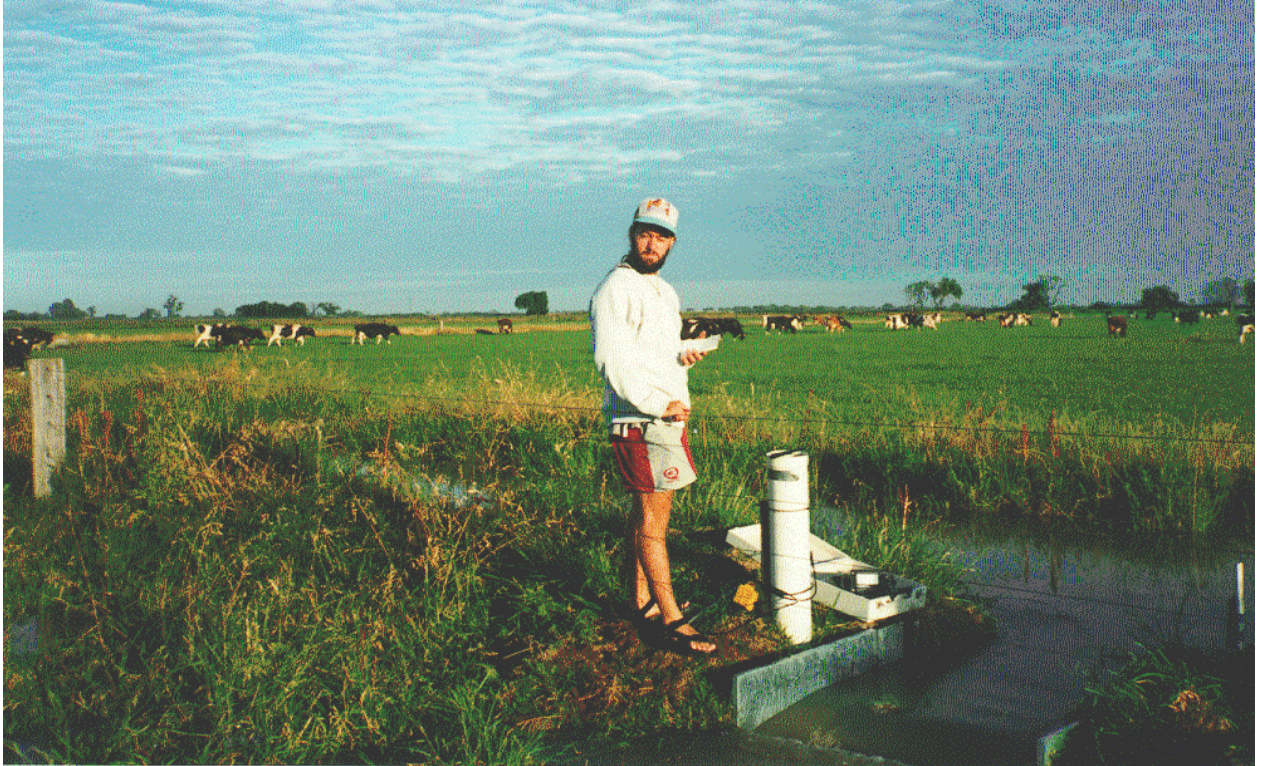
Photograph 1. A large rectangular flume was used to accurately measure the flow of supply water onto the bay during each irrigation event. For a given depth of water flowing through the flume, an accurate flow-rate can be determined.
