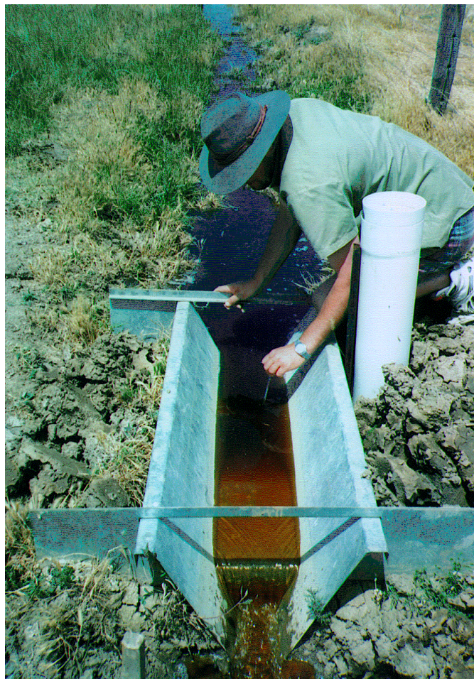
Photograph 2. Flow measurement flume in the monitored bay's drain. This type of flume can measure low flows accurately, making it ideal for monitoring small farm drains.
