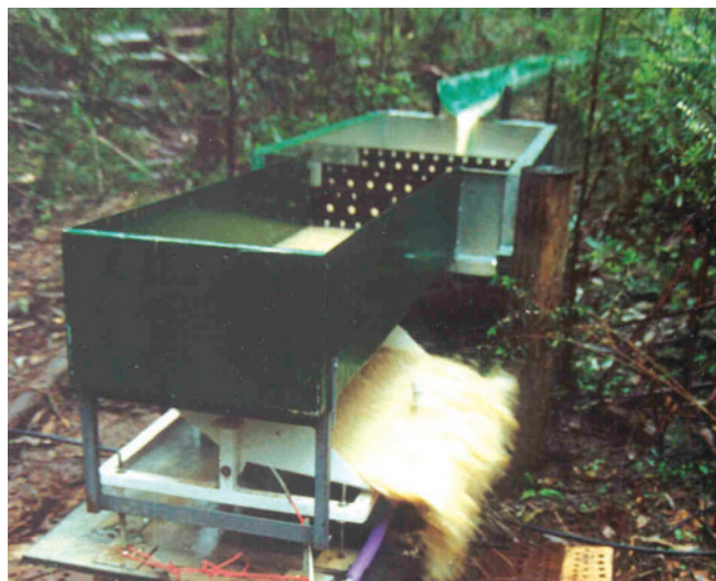
Figure 1. The experimental measurement apparatus during a storm event, showing delivery pipe from the road culvert, bedload trap, manifold, tipping bucket, and suspended load sampler (visible protruding from the discharging flow).
