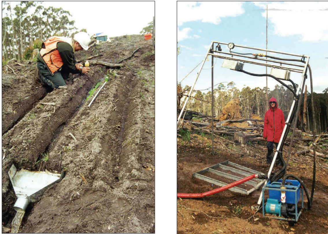
Figure 2. The runoff (left) and rainfall (right) simulation methods used to determine rill erodibility, interrill erodibility, and infiltration parameters.
